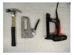
Figure 2 - NM cable installation tools
