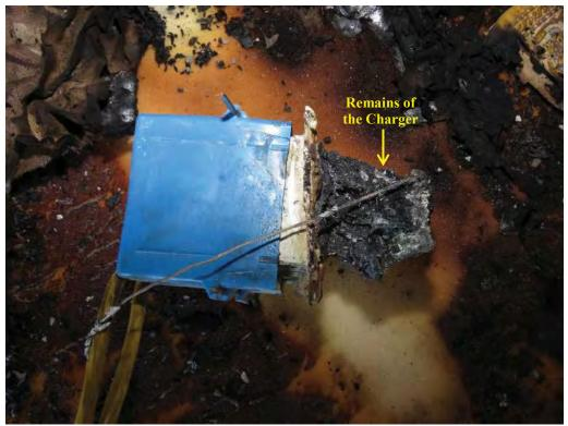
Photograph 8. 1-18-17 DLJ, IMG\_0068: The undamaged receptacle box seen after the receptacle was removed from the wall.
