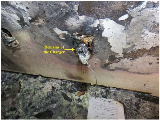
Photograph 6. 1-18-17 DLJ, IMG\_0052: A closer view of the damaged receptacle and charger.
