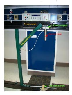
Figure 27 - Hammer impact simulator
