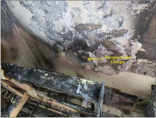
Photograph 5. 1-18-17 DLJ, IMG\_0048: The receptacle and remains of the charger.
