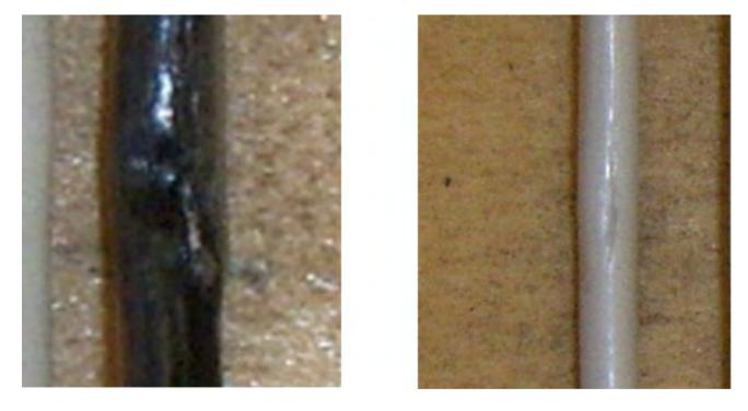
Figure 34 - NM Cable insulation cracked by 7ft-lb hammer impact
