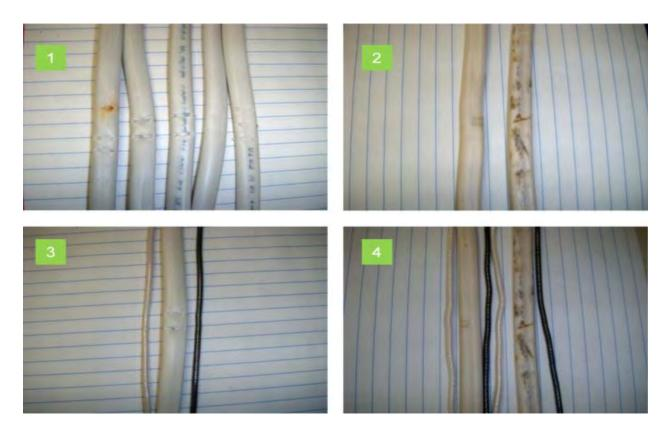
Figure 24 - Overdriven NM cable samples
