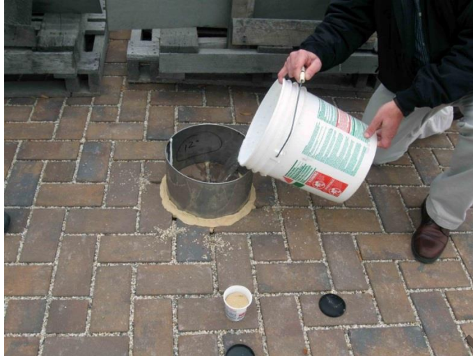
Figure 6-1. ASTM C1781 Test Apparatus to Measure Surface Infiltration.
