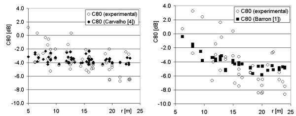
**Figure 1** – C80 vs r of experimental data and the C Model (Carvalho [4]), for  $V<18000\text{ m}^3$  (left) and the A Model (Barron [1]) for  $V>18000\text{ m}^3$  (right) for  $r < 23\text{ m}$ .
