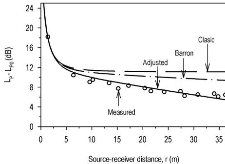
**FIGURE 1.** Sound pressure levels versus source receiver distance for the 2 kHz octave band in Sta Marina church.
