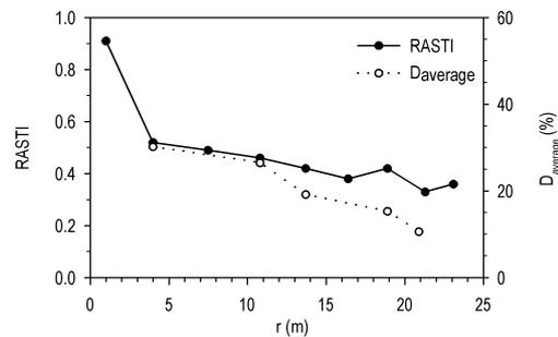
**FIGURE 3.** RASTI and  $D_{average}$  versus source-receiver distance in San Gil church.
