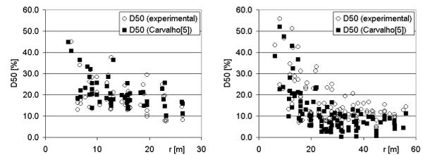
**Figure 2** – D50 vs r of experimental data and the C Model (Carvalho [5]) for  $V<18000\text{ m}^3$  (left) and  $V>18000\text{ m}^3$  (right)
