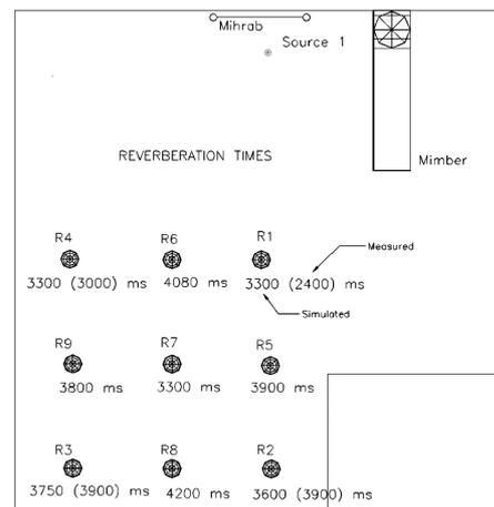
FIGURE 1. EDT of both measurement and simulation
