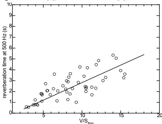
Fig 5 - Relation between reverberation time in churches and (volume/floor surface) ratio
