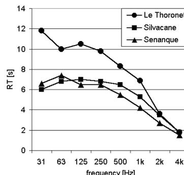
Figure 3. Reverberation Time (RT) versus Frequency
