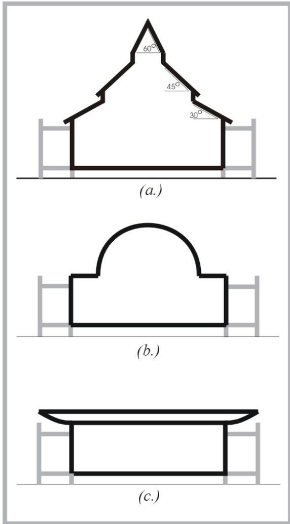
**FIGURE 1** : Basic roof shape, (a) pyramidal-tier roof, (b) Dome-roof, (c) flat-roof
