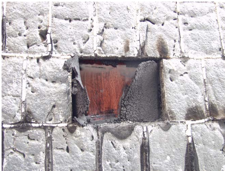
Figure 6. Pennguard wall after the ASTM E-119 test showing the condition of the primer coating of the steel plate
