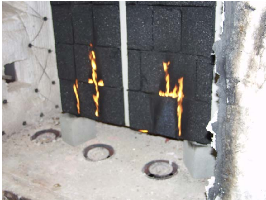
Figure 9. Flame propagation test after the burners were turned off
