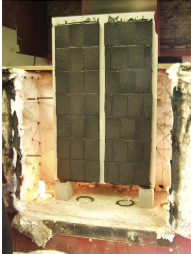
Figure 7. Two small wall sections of Pennguard lining mounted over the burners before the fire propagation test
