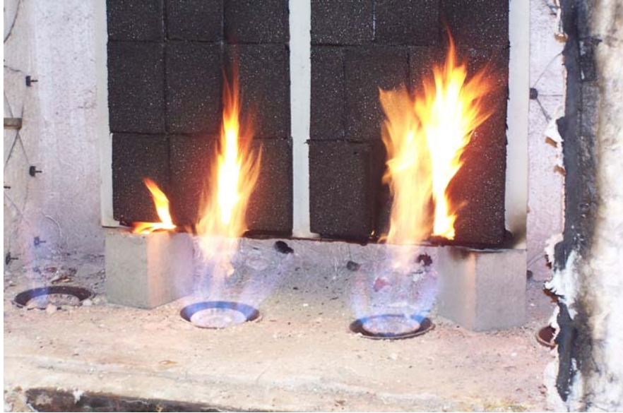
Figure 8. Flame propagation test with the burners on
