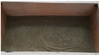
Figure 3. Test tank(Wooden box 1.6L X 0.5W X 0.6D m)
