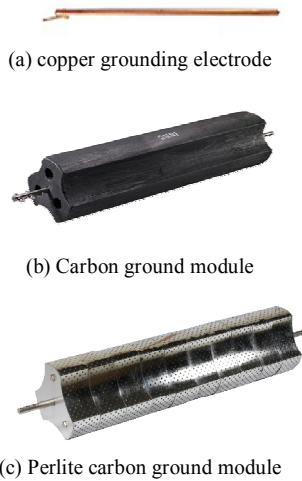
Figure 2. Test Samples of Grounding Electrode
