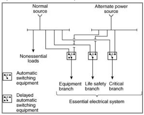
Figure Informational Note Figure 517.31(B)(b) Type 1 Essential Electrical System — Minimum Requirement (150 kVA or Less) for Transfer Switch Arrangement.
